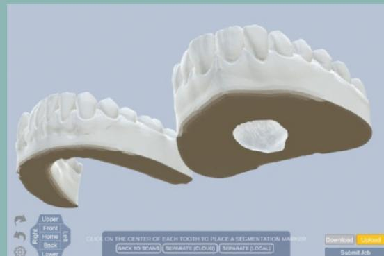
Fig 5-1-8 Capped upper and lower models during model preparation in the Archform software.
