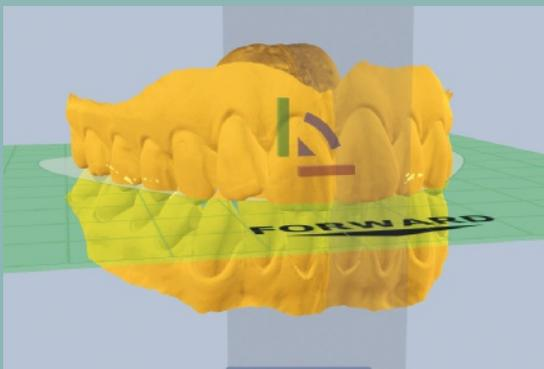
Fig 5-1-7 Model preparation module of Archform, showing the different planes used for model orientation with the option to tilt/translate the model in relation to these planes.
